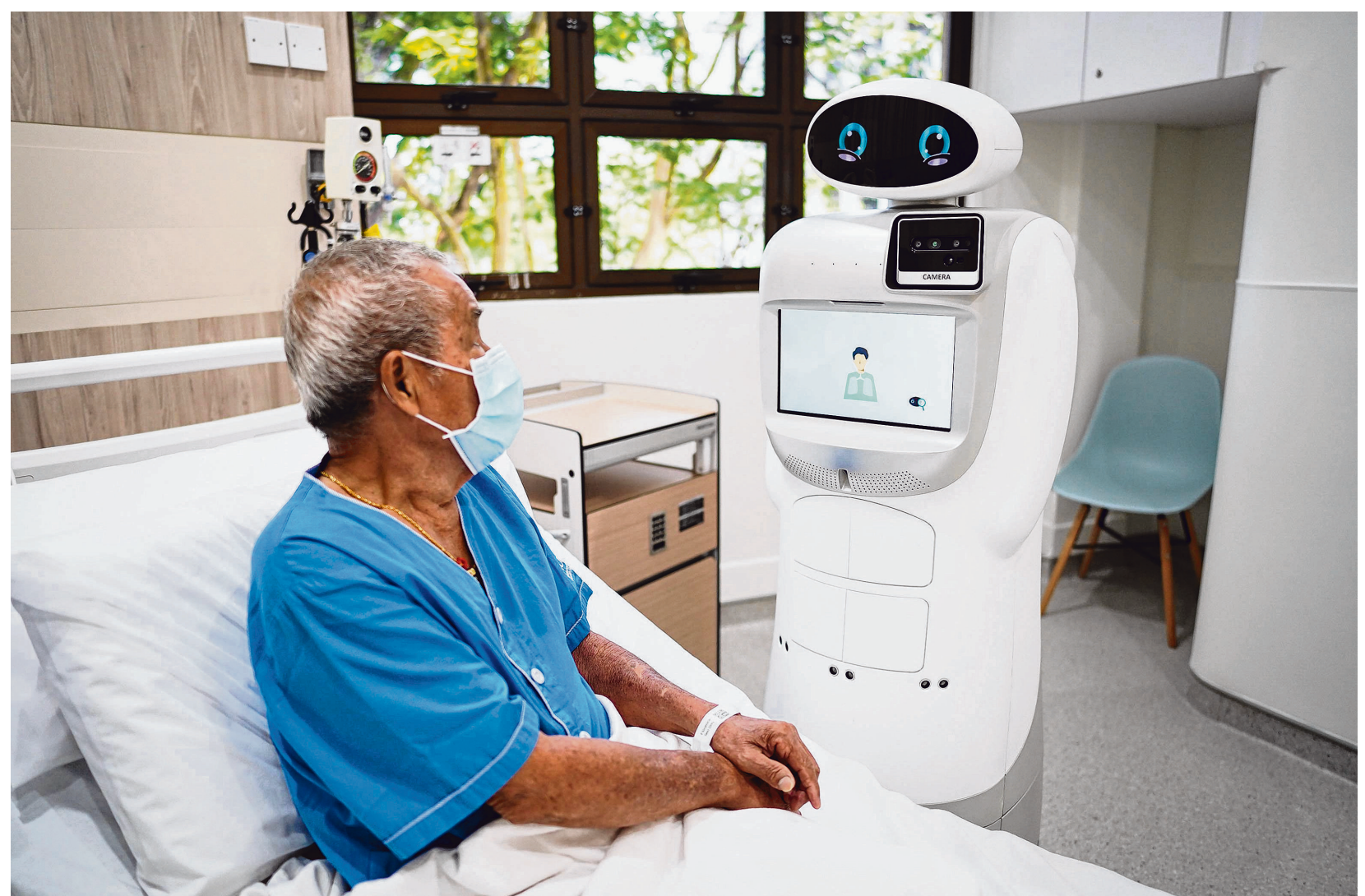
Florence the robot attending to a patient at Alexandra Hospital. It can identify a patient by scanning his wrist tag or with its artificial intelligence-based image recognition software, and is able to measure a patient's respiratory rate and other vital signs, among other things. ST PHOTOS: SYAMIL SAPARI
