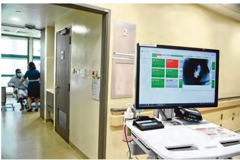
The smart predictive patient monitoring system at TTSH uses thermography, machine learning and predictive algorithms to predict when a patient is getting out of bed, giving nurses time to intervene. ST PHOTO: DESMOND WEE
