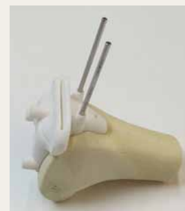
⚡ An example of the 3D printed Patient Specific Instruments (PSI) being fitted onto the distal femur.
