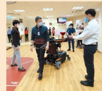
Showcasing the Mobile Robotic Balance Assistant (MRBA), a transformable robotic wheelchair which prevents falls and enables patients to safely practise walking, and participate in daily living activities in home and institutional settings.
